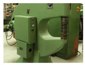
Capacities Steel: 6 mm lightmetal: 8 mm Stainless steel: 4,5 mm
